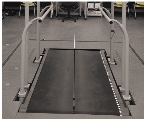
Figure 1 : Image from the Neuromechanics Laboratory of the University of Colorado Boulder showing a split-belt treadmill.
